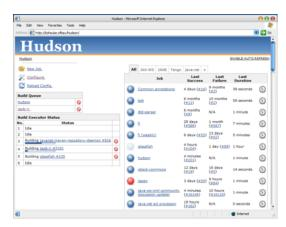
Example of output from a Continuous Integration tool
