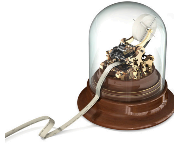
Figure 5. A ticker tape machine
