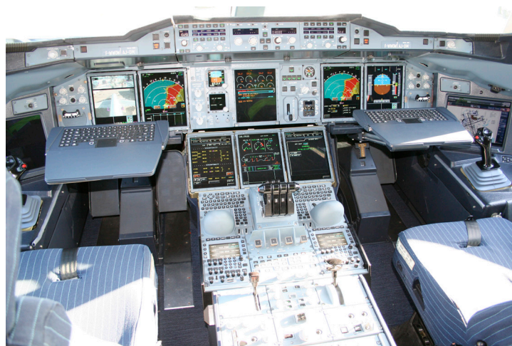
Figure 14. The cockpit of an AirBus A380 with the side-sticks
