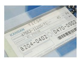
Figure 3. A Toyota kanban colour-coded card
